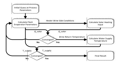
Each of the boxes are explained in detail below, along with applicable thermal models used. What is not shown is that the user defines the operating conditions used to evaluation each simulation. A batch input file is used for this purpose and a sample is shown below.
